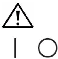
The power supplies for the TriPlus RSH/TriPlus 100 LS, the Temperature Controlled Drawer have the symbols I/O on the label for the power switch to indicate ON/OFF.
